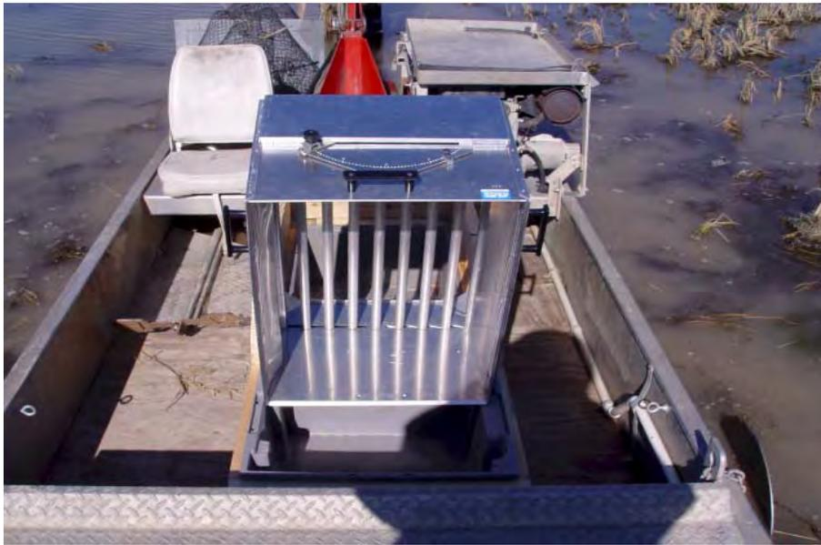
Figure 2. Size grading of crawfish was accomplished in the boat at harvest with a variable fish grader. Grader was adjusted for different size categories.
